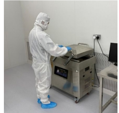
Double vacuum bagging
